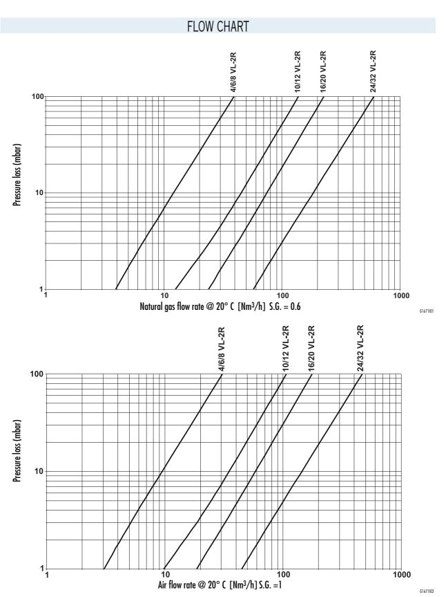
The capacities are reffering to the shaft of the secondary regulation completely open.
