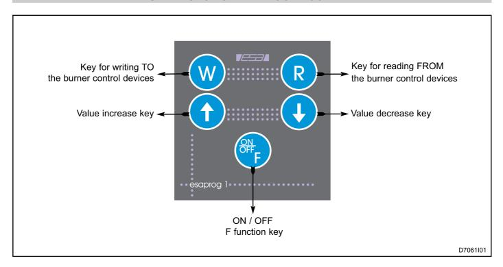
ESA PROG-1 diplays in automatic mode the available menus to which you can enter with the function key. In the "ADDRESS" menu the display indicates both the parameters of the address and if the change phase is activated a flashing point indicates the data that can be changed with the arrow keys. During the communication with the flame control device it indicates the operation taking place (reading or writing). In the other automatic
