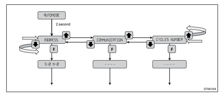
When communication mode is selected via the "ECS BY WIRE " cable (see programming mode), the SEND COMMAND menu also appears. In this menu there is a com-
