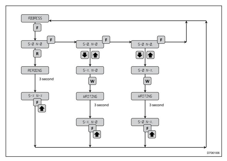
To enter the menu press the "F" key. Press it again to select the change of segment S (with decimal point flashing) and with the increase and decrease keys set the new value. After having edited the new segment (the decimal point remains flashing) writing with the "W" button can be carried out. If not, press the "F" key proceeding with
