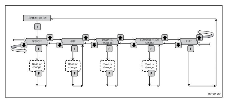
The SEGMENT and NODE parameters allow to individually edit each segment or node of the serial address. The BAUD RATE PROTOCOL parameter allows to select the speed and type of serial communication of the burner control device. The ESA burner control device standard is 4800 b/s ECS. Below we have indicated the possible speeds and communication protocol available on the flame control devices. Furthermore we annotate that ESA
