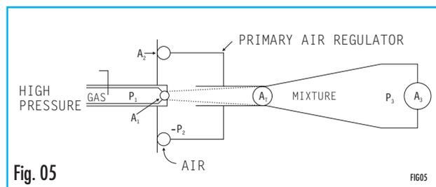
the remaining 20 % of air will be utilized as secondary air to be supplied to the combustion system with a specific draft in the combustion chamber. The latter though is not very important as far as the effects of the assessment of the capacity limits of the mixers is concerned.
