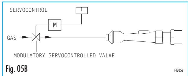
pressure switch) servocontrolled valve on the gas line. It is however necessary to pay much attention when choosing and installing the control. It is important to remember that this type of regulation can only be used at high pressures and gas capacities. The use of the modulatory regulating system is recommended for pressures of at least 3,000 mm H<sub>2</sub>O.
